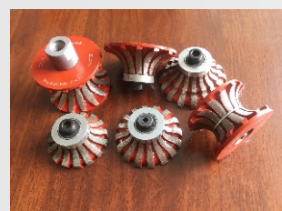
Segmented router bit
